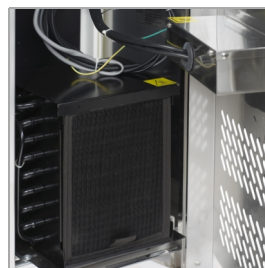
Easy access to clean dust filter
